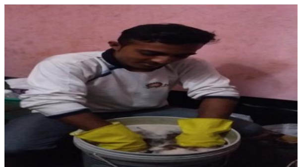
Fig 1: Treatment of Coir with NaOH
