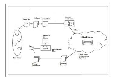
Fig -1: System Architecture of proposed system
