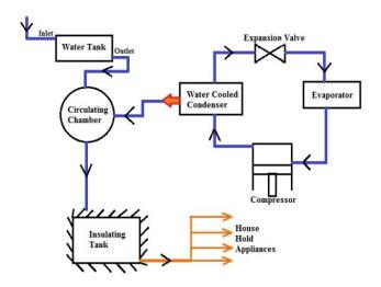
*Fig. 9:* Flow chart for working of AC integrated Hot water system [16]
