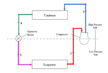
Fig. 1: vapour compression refrigeration cycle [4]
