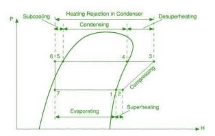
Fig. 2: P-h diagram with sub-cooling and super heating [4]
