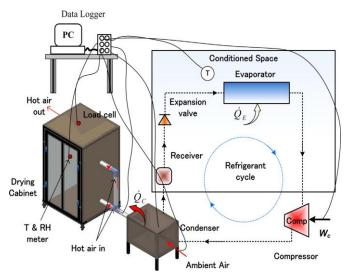
Fig. 6: RAC, experimental apparatus, and data acquisition unit. [14]
