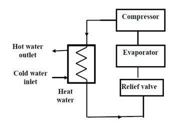
Fig. 10: Diagram of the modified refrigerating circuit to heat water [19]
