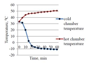
Fig. 8: Temperature-Time plot (without load) [6]
