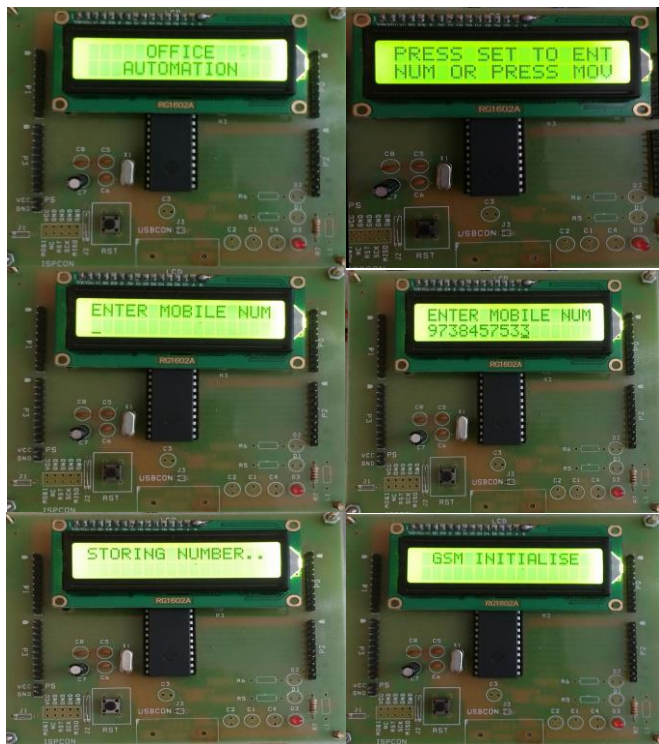
Fig 3: Shows the Hardware Assembly and its Initialization, displayed on an LCD.
