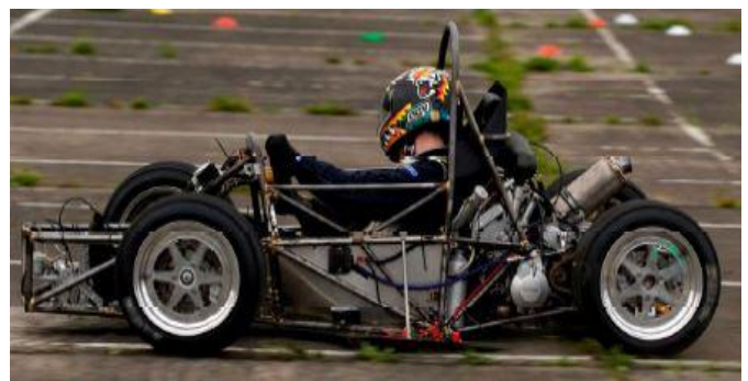
Fig-1: FSAE Vehicle with 600cc engine in rear
