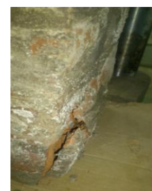
Corner Crushing of Brick of 5-Layer Red Brick Prism
