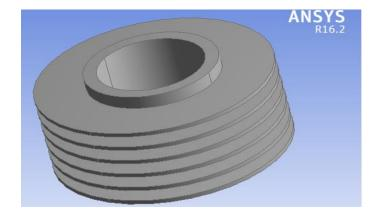
Fig-2: Model of cylinder with Rectangular Fins.
