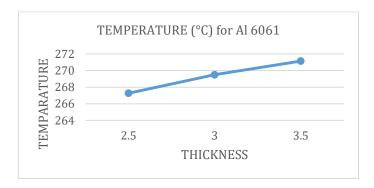
**Fig-8:** Graphical representation of temperature Distribution results with ANSYS for Rectangular Fins of Aluminum Alloy 6061 with variable size fin thickness.
