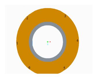
Fig-3: Placement of thermocouples.
