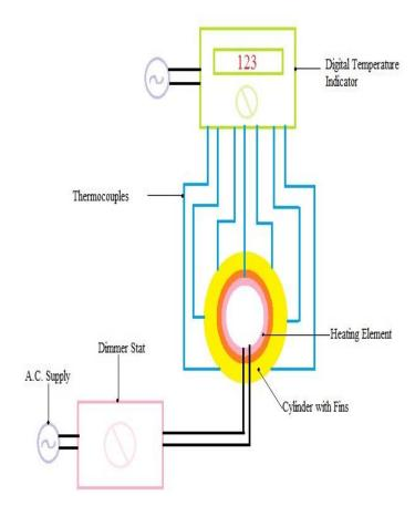
**Fig-4:** Experimental setup for measurement of temperature at tip of the fin.
