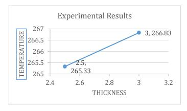
**Fig-9:** Graphical representation of temperature Distribution results with Experimental Model for Rectangular Fins of Aluminium Alloy 6061 with variable size fin thickness.
