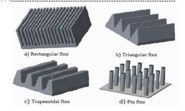
Fig-1: Different types of fin geometries
