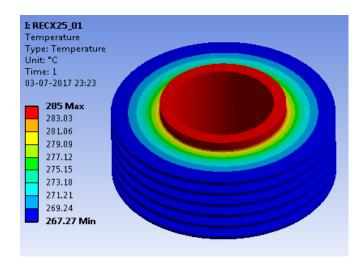
**Fig-6:** Temperature Distribution for Rectangular Fins of Aluminium Alloy 6061 with 3.0 mm Fin Thickness
