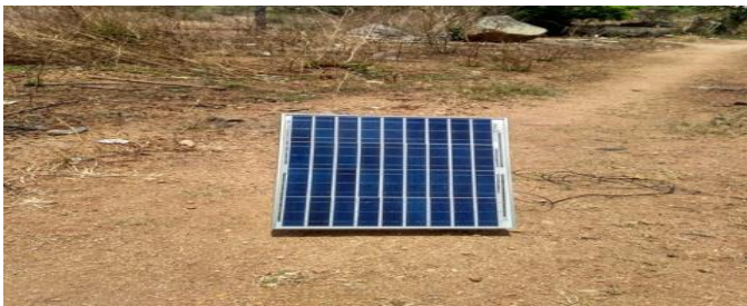
Fig.2. A 30Wp off Grid Solar Roof Top Photo Voltaic cell
