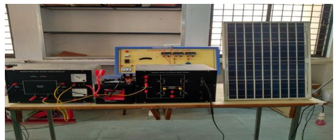
Fig 4. The real time module of 30WP Solar Roof Top Power Plant
