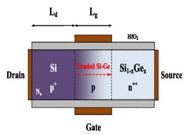
Fig-8: Structure of Hetero-junction TFET [21]
