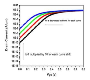
Fig-2: MOSFET Transfer characteristics with reduction in  $V_T$  [5]
