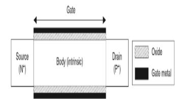
Fig-4: Schematic of p-channel Double Gate TFET [19]
