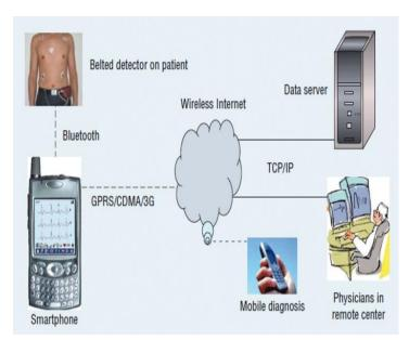
Fig -2: A typical remote diagnosis model
