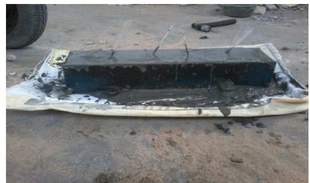
Fig. 13: Finishing Of Prism
