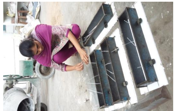
Fig. 11: placing of fibers
