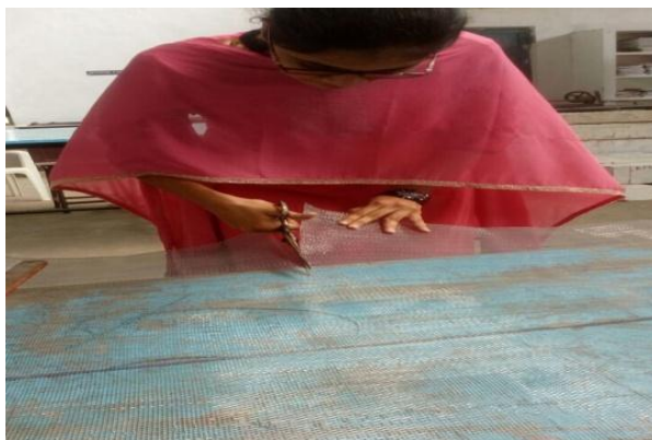
Fig.9: Cutting Wire Mesh
