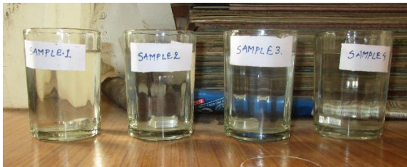
Fig.2: Specimens exposed to 3.5% NaCl solution for a period of 28 days.
