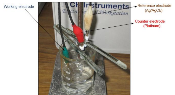
Fig.3: Setup of three electrode flat corrosion cell.
