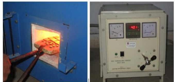
Fig.1: Carbolite furnace at 400°C for annealing heat treatment at NIFFT Ranchi.
