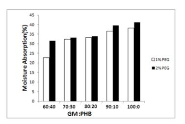
FIG.4. Moisture absorption of blend films at various compositions
