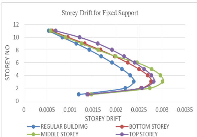
Chart 4 Comparison of Storey Drift for Regular and Mass Irregular Building for Fixed Condition
