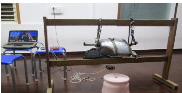
Figure 3.1 Experimental set up for LMS Impact testing
