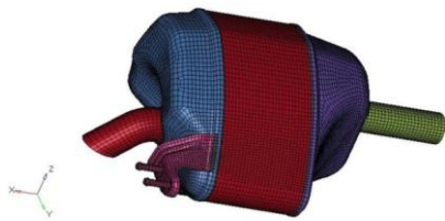
Figure 2.4 Meshed Model of Muffler
