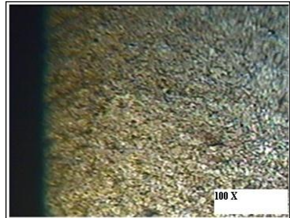
Fig:4.2.a Specimen microstructure with un tempered Martensite
