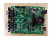
Figure 7: ARM7 Microcontroller Board
