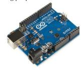
Figure 3: Arduino Uno Board
