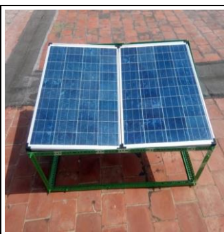
Figure-4: Solar Panel (75W, 2Nos) used for SPADIS
