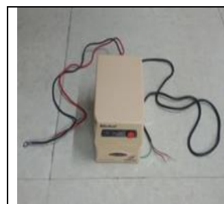
Figure-6: Inverter (250VA/12V) used for SPADIS
