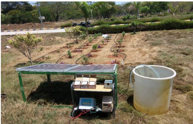
Figure-16: Solar Powered Automated Drip Irrigation System
