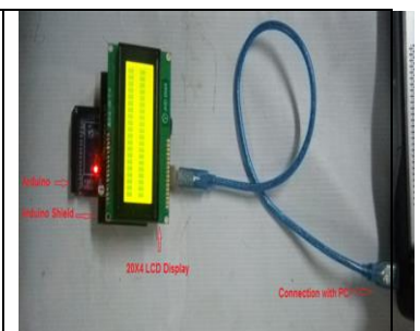
Figure-15: LCD display connected with Arduino
