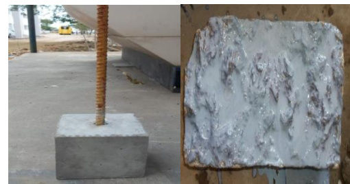
Fig -1: Pullout Specimen & Bonding of Repaired Concrete Using Polymer
