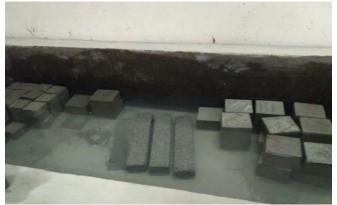
Fig. 1.2.2Curing tank of cubes and prisms
