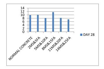
.Tab.2.7 Graph showing flexural strength (N/mm<sup>2</sup>)
