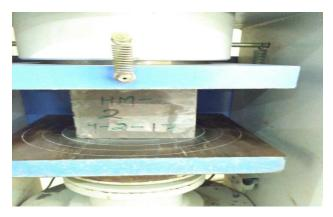
Fig.2.3 Cube placed in testing appartus
