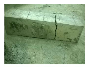
Fig.2.6 Prism after testing
