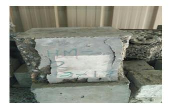
Fig.2.4 Cubes after compression testing
