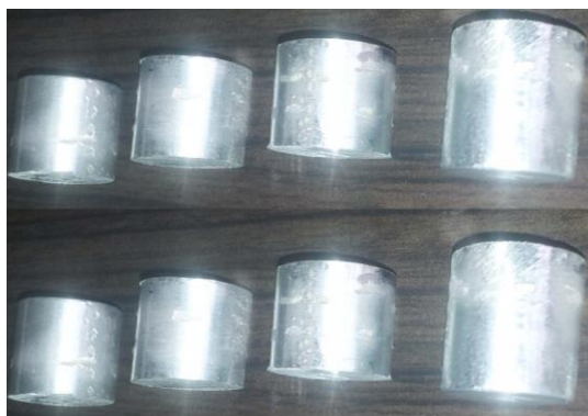
Fig. 6 Specimen for roughness measurement after turning
