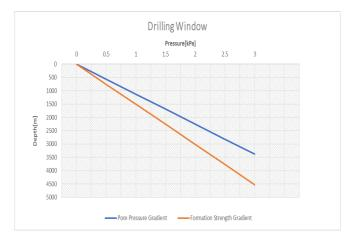
Figure -1: Drilling window
