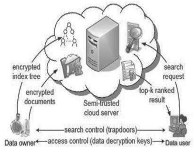
Fig 1. The architecture of ranked search over encrypted cloud data. Advantages of Proposed System:
