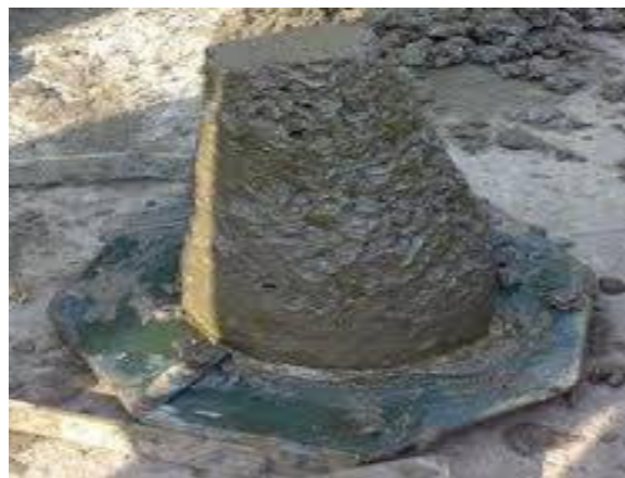
Fig 4. Sample of concrete mix for Slump Test
