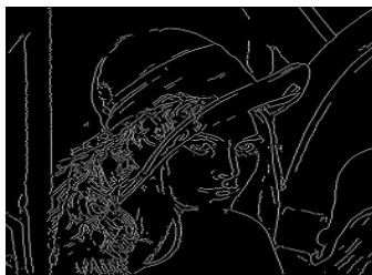
Fig-3: Canny Edge Detection with 9x9 mask and \sigma=1.4
