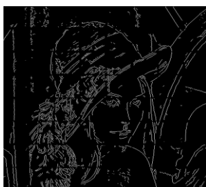
Fig-4: Applying original canny algorithm on block Guassian noise of 9x9 with \sigma=1.4
