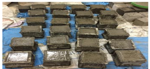
Fig 10 –moulds used for casting specimens.
