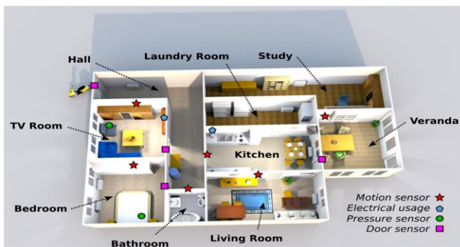
Fig -4: Normal House with Install Sensors
