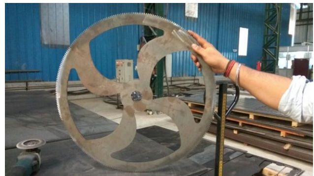
Fig.11 Sprocket after Laser Cutting
