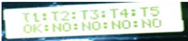
Fig 2. Track Status on LED Screen
