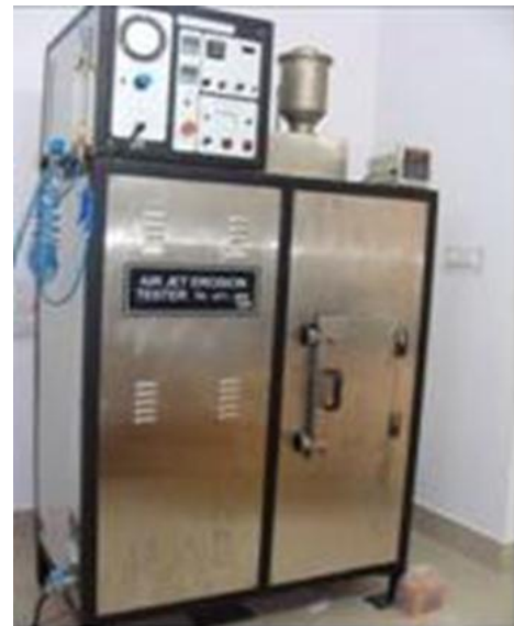
Fig. 1(b): Solid particle erosion test set-up
