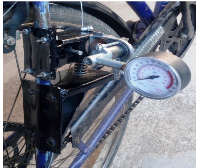
Fig. 2 Compressor with supporting structure
