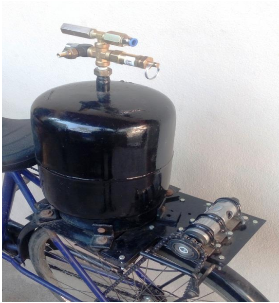
Fig. 4 Air Receiver, Air Motor Frame
