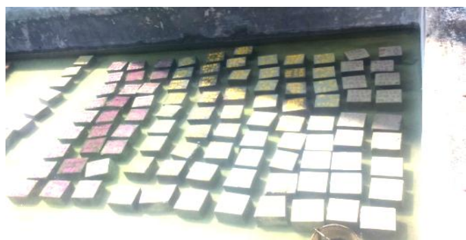
Fig-3: Curing of Concrete Cubes
