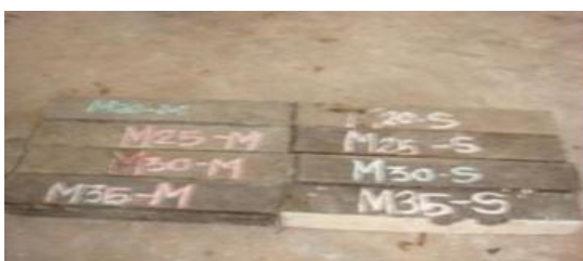
Fig -2: Specimen for flexural strength testing
