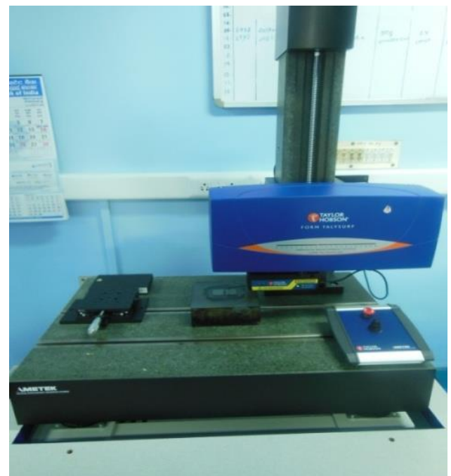
Figure 3: Experimental setup for measurement of surface roughness
