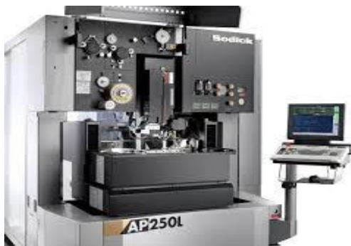
Fig1 : wire cut EDM machine
