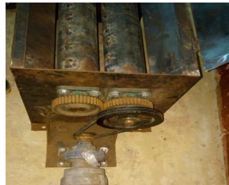
Fig 1 Gears and Belt driven mechanism
