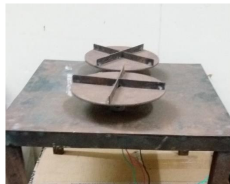
Fig 2 5v dc motors with coin dispersive mechanism
