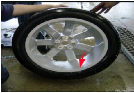
Figure showing Max deformed area where when there will be air leakage (tube less tyres) from the tyres
