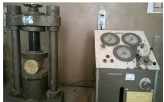
Fig. 2 Split tensile strength test
