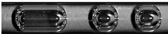
Fig-3: Taylor-bubble flow inside a capillary tube [Khandekar, 2010]
