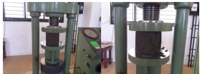
Fig-3: Compressive strength test before failure & after failure
