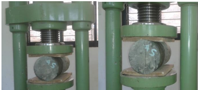
Fig-4: Tensile strength before failure & after failure
