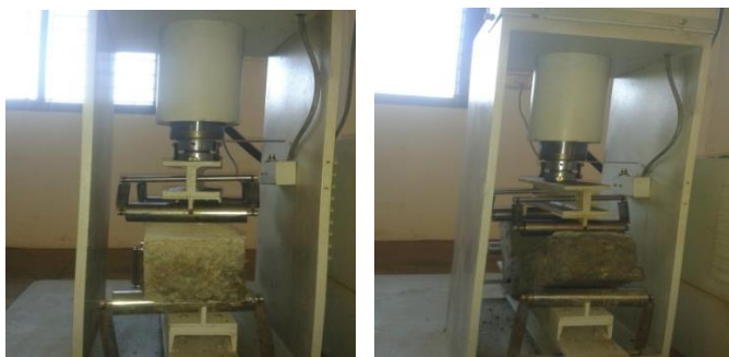
Fig-5: Flexural strength before failure & after failure
