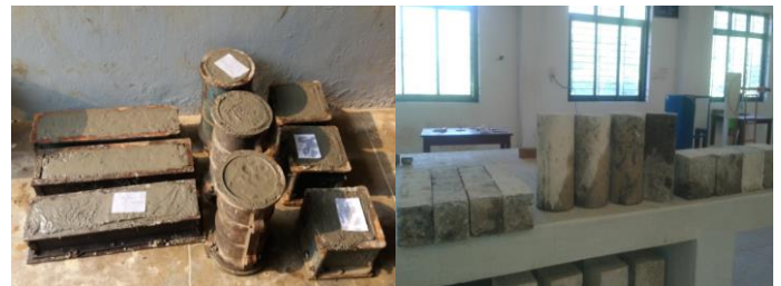
Fig-2: Casted specimens & Demoulded specimens
