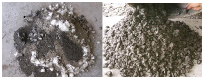
Fig-1: Mixing of all materials, dry mixing & wet mixing
