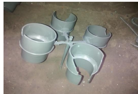
Fig2A.Defects in pressure reducer Part
