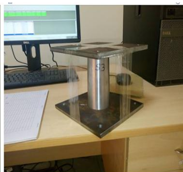
Fig.5. Al cone embedded in Steel plates
