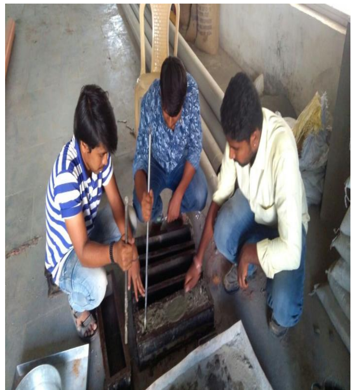
Figure 5.6: finishing of moulds
