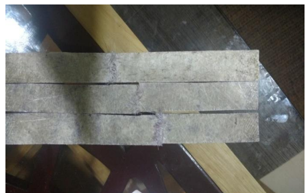
Fig-3: Prepared tensile test specimen with 80% glass fibre and 20% resin
