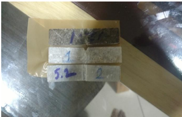
Fig-4: Prepared impact test specimen of glass fiber
