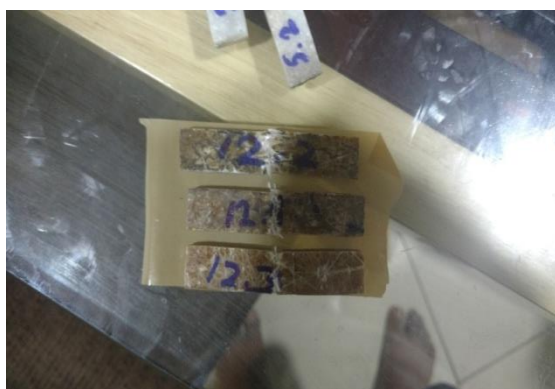
Fig-5 : Prepared impact test specimen of glass fiber
