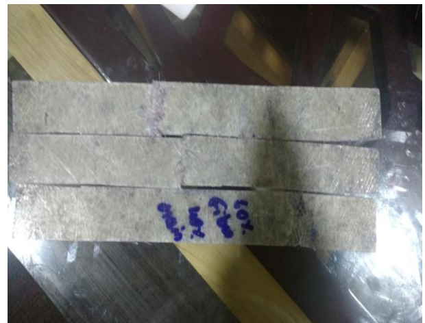
Fig-2 : Prepared tensile test specimen with 60% glass fibre and 40% resin
