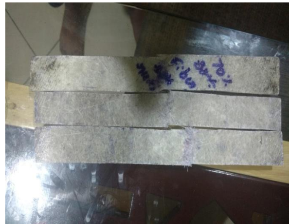
Fig-1: Prepared tensile test specimen with 70% glass fibre and 30% resin
