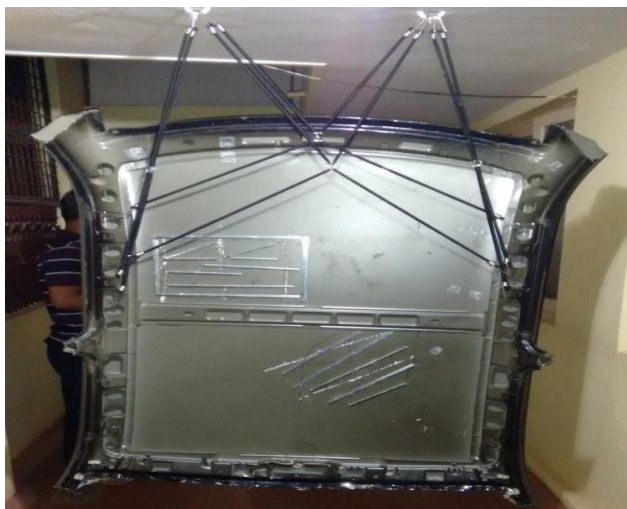
Figure.16. The roof component hanged freely using hangers with stiffener
