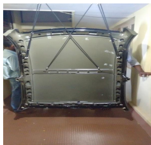
Figure.14. The roof component hanged freely using hangers without stiffener
