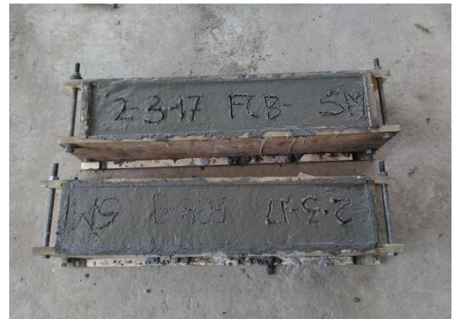
Figure 7. Casted Ferrocement Concrete Beams
