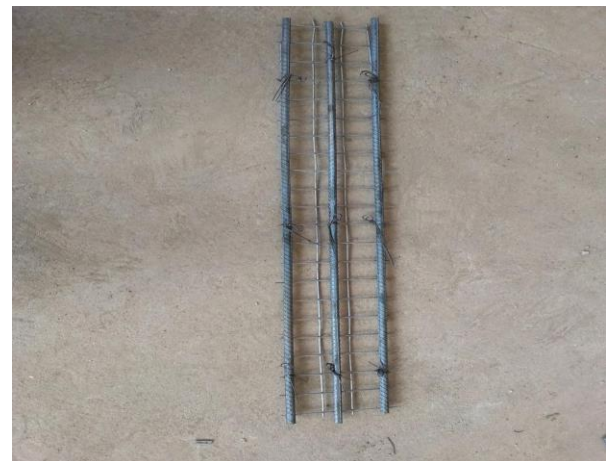
Figure 3. Reinforcement Used in Conventional Ferrocement Beams
