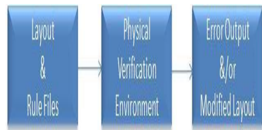
Fig -1: Physical verification top view [8]
