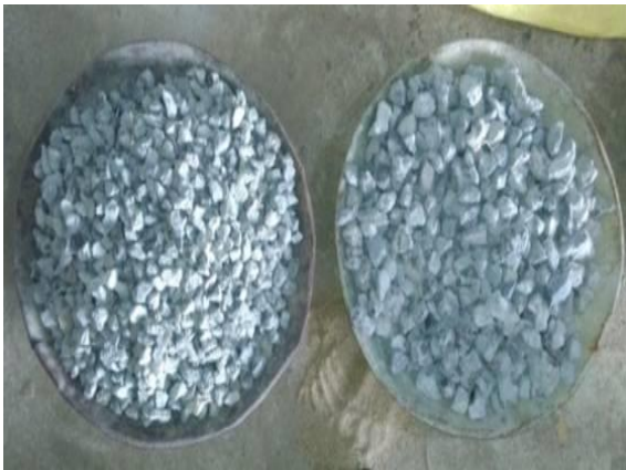
Fig. 1. Demolished Concrete Aggregate
