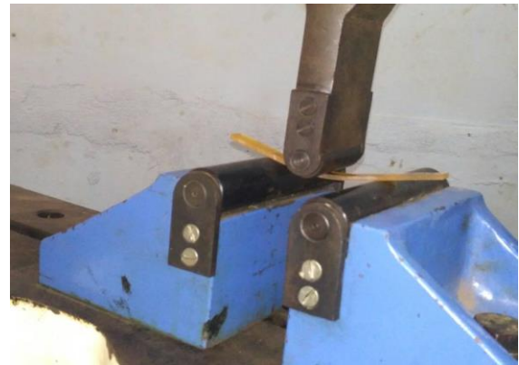
Fig - 2 Specimen loaded for testing
