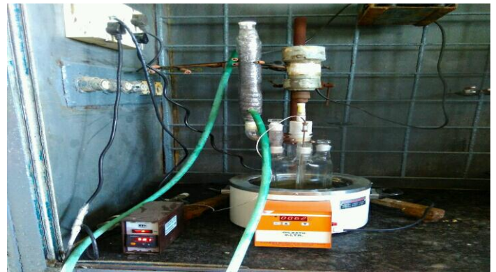
Fig-7: Water Extraction Kettle
