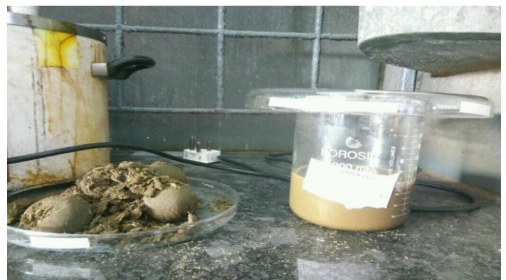
Fig-8: Cake and filtrate separated from extracted mass
