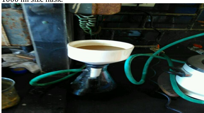
Fig-11: Vacuum filtration of ethanol extracted mass
