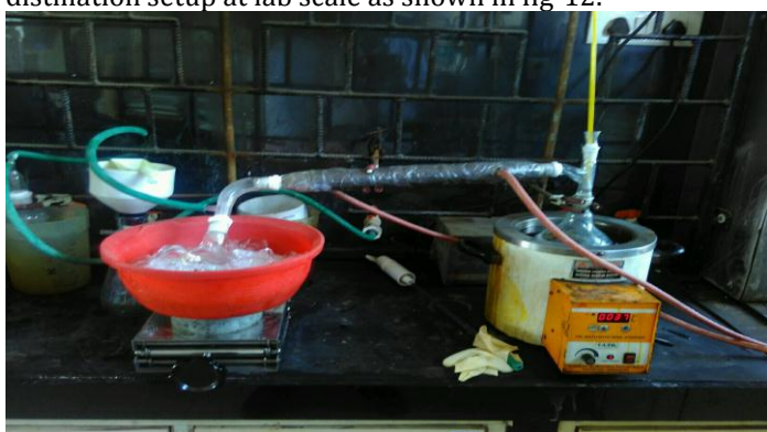
Fig-12: Concentration of mimosine supernatant by using vacuum pump
