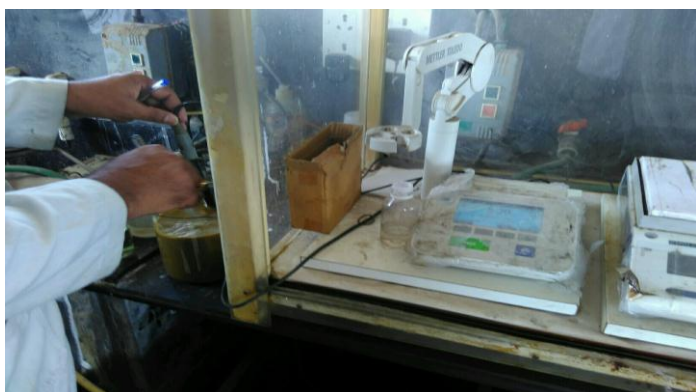
Fig-10: pH adjustment by pH meter
